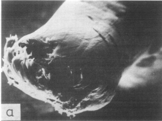
Figure 8 Fracture surfaces of PE fibres under strain exposed in an \text{NO}_x environment. Samples were held at (a) 70% strain for 20 min, and (b) 90% strain for 20 h at room temperature. Magnification: (a) 220x, (b) 110x
